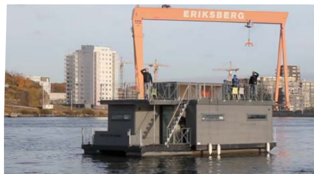
Ocean Living Motor: 2xGS18. Batteri: Bly 48V, 800 Ah Prestanda: 3 kn - 7 h, 4 kn - 1 1/2 h
