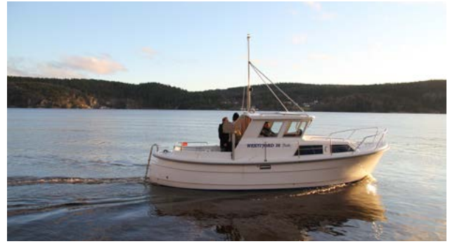
Westfjord 26 , Motor: 2xGS10. Batteri: Bly 24V, 200 Ah Prestanda: 4 kn - 6 h, 5 1/2 kn - 30 min
