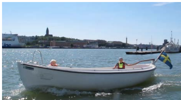
Vikensnipa , Motor: GS10. Batteri: Litium 24V, 200 Ah Prestanda: 4 kn - 11 h, 6 kn - 1 1/2 h
